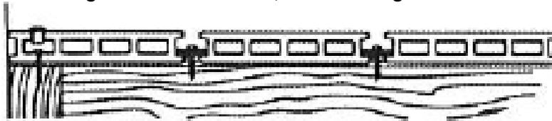
**Figure 4 – Slide & Go® Hidden Fastener**
