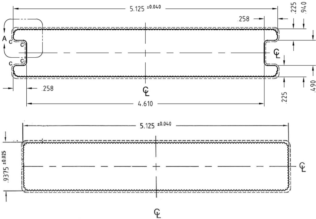
**Figure 3 – Enviroboard, Grooved Edge Installation**
