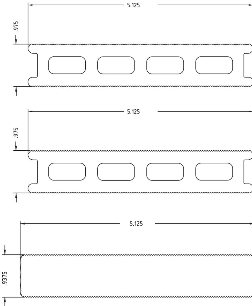
**Figure 2 – TRUNORTHDECK™ Composite Deck Boards – Co-Extruded**
